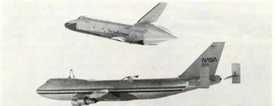
The explosive bolts are fired and astronauts Fred W. Haise and C. Gordon Fullerton begin their powerless descent glide.
